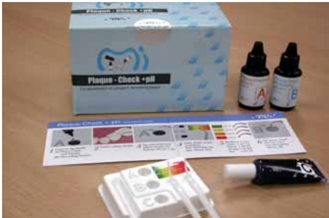
Figure 1: The Plaque-Check+pH kit for testing plaque fermentation (GC Corporation, Japan) uses a colourimetric method to demonstrate the pH drop of the Stephan curve when intact plaque is challenged with sucrose.
