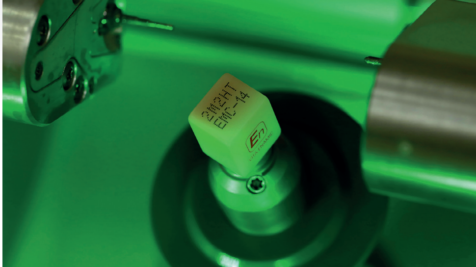
Figure 8: The highly translucent, hybrid ceramic block in shade 2M2 positioned in the grinding machine
