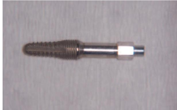
**Figure 12: Osstell smart peg (type 47) fitted to Dio implant.**
