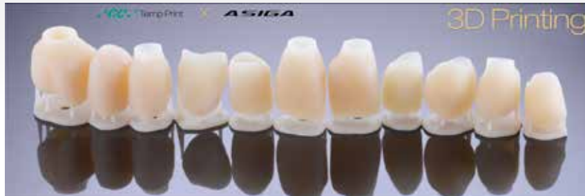
Figure 13: Second set of provisional restorations printed with GC Temp PRINT (medium shade) using the Asiga Max UV 3D printer.
