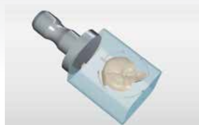
Figure 7: Once happy with your design, position the sprue on your restoration to a favourable position.
