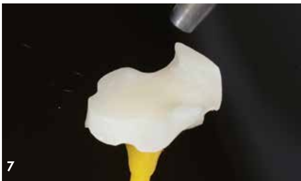
Figure 7: Air-blasting the bonding surface with 50 – 100 µm aluminium oxide at 1 – 1.5 bar; followed by cleaning.
