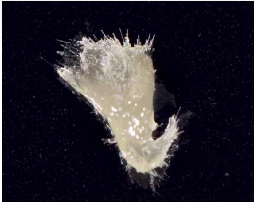
Figure 2: The unique size of the short fibres is visible when the SFRC material is extruded from the unitip.
