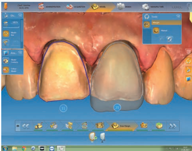
Figure 7: The design of the hybrid ceramic veneer in the Cerec software.
