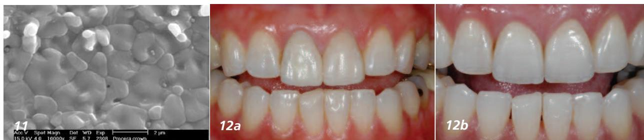
**Figure 11:** A scanning electron micrograph of the microstructure of an alumina ceramic.
