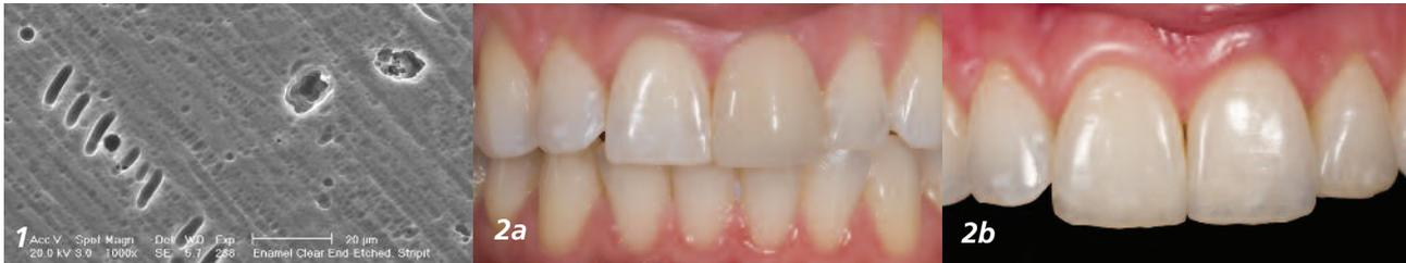
**Figure 1:** A scanning electron micrograph of the microstructure of a glass veneer porcelain.
