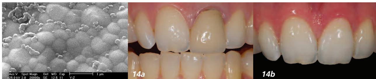
**Figure 13:** A scanning electron micrograph of the microstructure of a zirconia ceramic.
