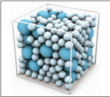
Figure 1: Bi-modal filler size distribution for optimal filler load.
