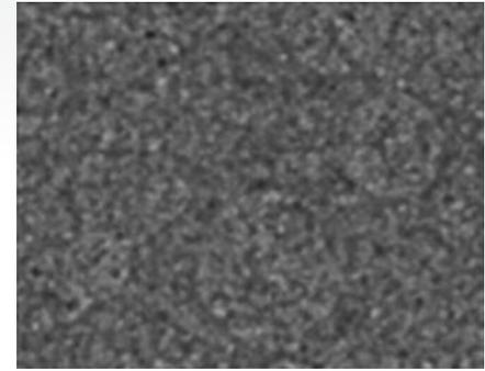
Figure 3: SEM picture of an abraded surface of ceram.x SphereTEC with homogeneously embedded (hardly visible) SphereTEC filler particles (Latta, 2015).
