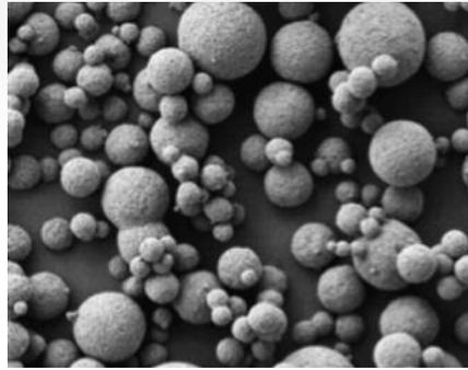
Figure 2: Typical SEM-pictures of SphereTEC fillers (Hagner, 2014).
