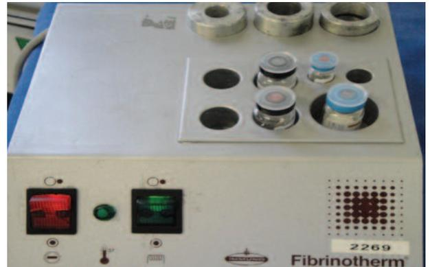
**Figure 8:** The Fibrotherm will guide the 4 tubes to the ambient temperature (37°C) by using a thermostated agitator.
