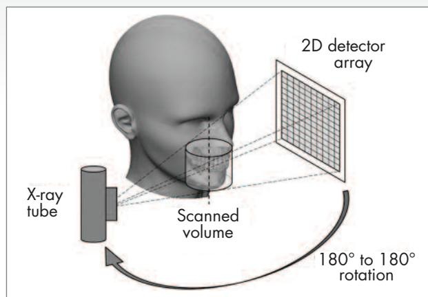
Figure 4: The x-ray source and reciprocating image detector synchronously moves 180° to 360° around the patients head.
