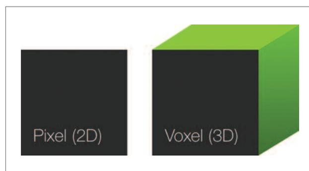
Figure 10: Pixel is the basic 2D basis image picture element, whilst a voxel is 3D picture element and thus represents the smallest individual volume element of a 3D scan.
