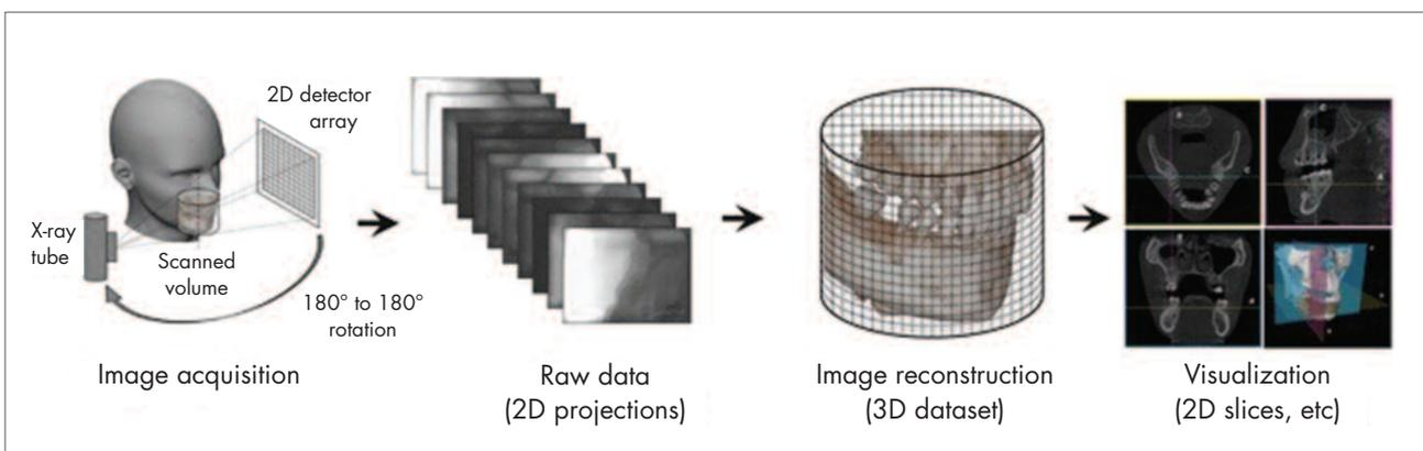
Figure 9: Image workflow stages of a 3D CBCT scanner.
