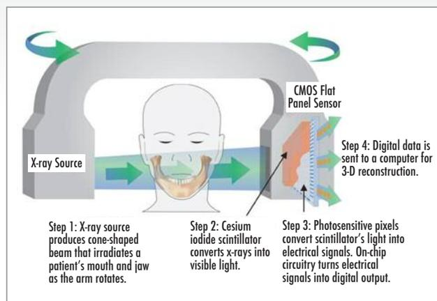
Figure 3: Conversion of in-coming X-ray photons to an electrical signal by the image detector.
