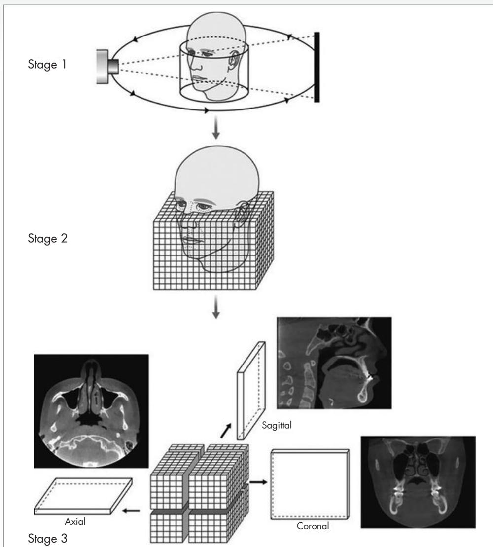
Figure 11: The 3D volumetric data set is a compilation of all available voxels presented to the clinician (Stage 2) and presented to the clinician in real time on screen as secondary reconstructed 2-D cross sectional images in three orthogonal planes (axial, sagittal and coronal) (Stage 3).
