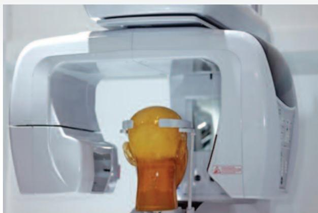
Figure 1: Basic elements of CBCT imaging hardware – X-ray source on the left, Image detector or sensor on the right, and the gantry or rotating platform that connects the x-ray source and the detector.
