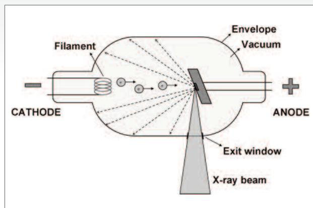
Figure 2: Basic elements of a CBCT X-ray source.
