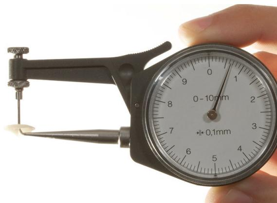
**Fig 5** The pressed veneers are approx. 0.6 mm thick.
