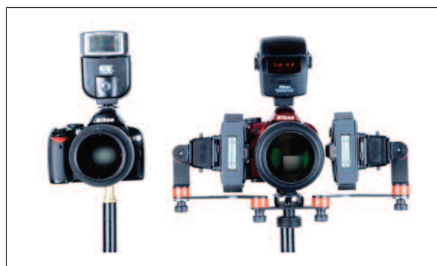
Figure 4: Different setups for obtaining cross-polarised photography. Left: a single flash with a polarised niter on the camera. Right: a twin flash using two polarising niters. Both options always had a polarised niter adapted in front of the lens
