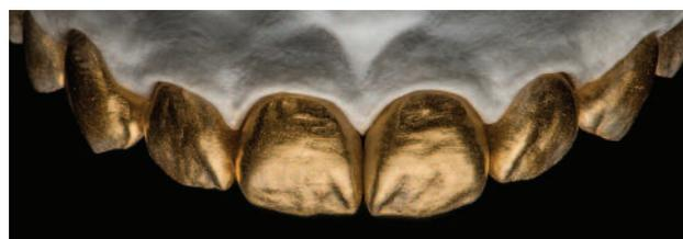
*Fig. 11: Evaluation of the surface morphology with the help of gold powder*
