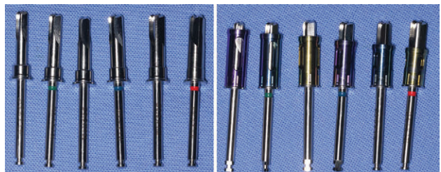
Figure 3: On the left the drills can be seen without any stoppers and on the right the stoppers from left to right increasing the drilling depth in 1mm increments from 2mm to 7mm.
