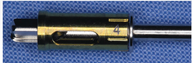
Figure 2: The stoppers fit on all the instrumentation and the depth is shown on the stopper (in this case 4mm limiting the drilling depth to 4mm)
