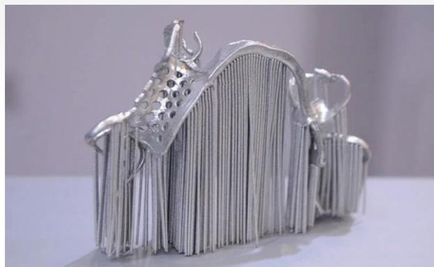
Figure 4: SLS 3D printed metal partial denture framework in CoCr
