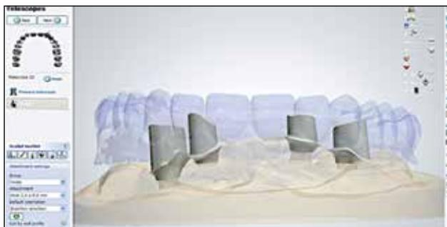
Figure 8: Reconstruction of the primary structure after scanning the model, abutments and set-up.
