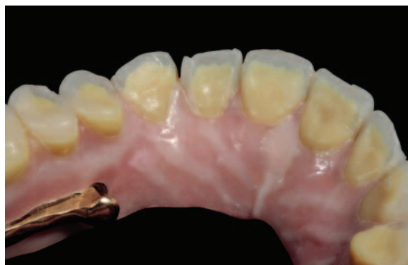
Figure 1: Removable implant-borne bar-latch prosthesis with conventional PMMA denture teeth after a service life of two years. High chewing forces and poor wear properties resulted in the rapid damage of the occlusal surfaces.
