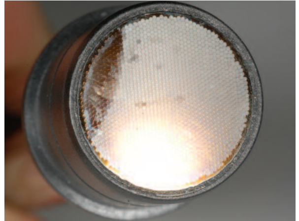
Figure 6: Defective light guide. The dark fibres are no longer capable of transmitting light.
