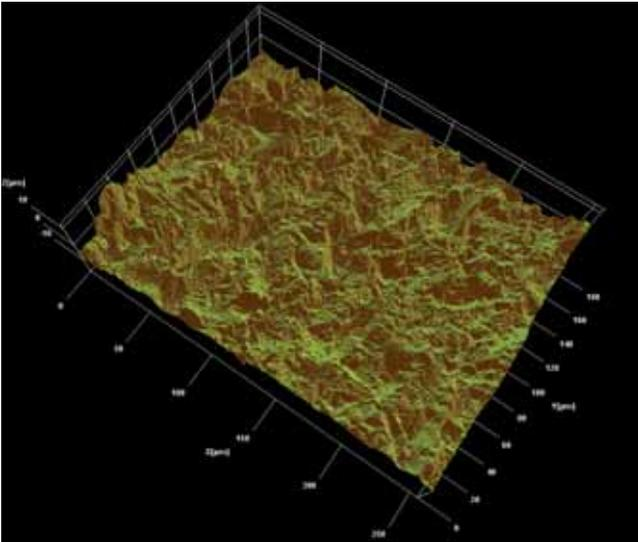
Figure 2a: Digital image from a surface roughness measurement of an OsseoSpeed™ flank area, 200 x 264 μm. The surface has  $S_a$  approximately 1.5 μm and Sdr 50%; a roughness found to be optimal for bone anchorage in previous experimental studies.
