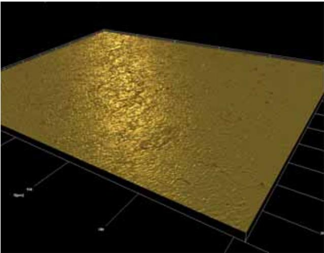
Figure 2b: The nanometer roughness of the OsseoSpeed™ surface;  $S_a$  of 22 nm and Sdr of 1%. The nanometer roughness may be important for early protein adhesion and consequent enhanced bone formation around the implant.
