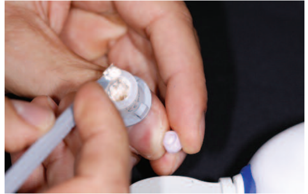
Figure 22: When exposed to vibration, IPS e.max Crystall./Connect becomes liquid.
