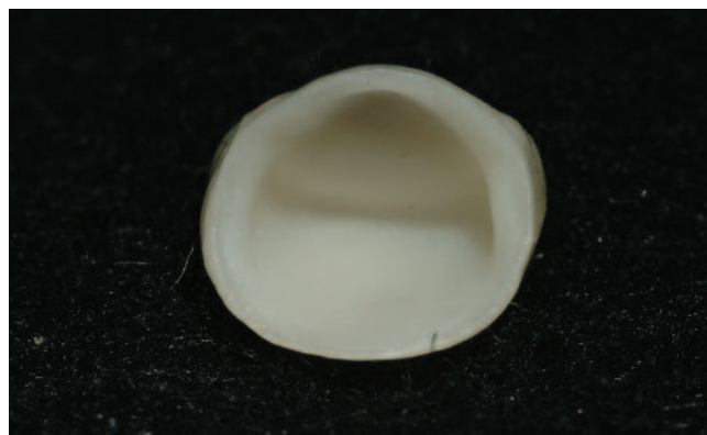
Figure 13: Well etched, clean, internal surface after removal of white precipitate. Compare with Figure 11
