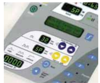
Figure 4: Instrument panel for settings on a ErCrYSGG hard tissue laser.
