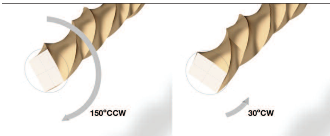
Figure 4: The WaveOne GOLD file engages 150 degrees CCW and 30 degrees CW, turning 360 degrees after three cycles of reciprocation.
