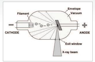
Figure 2: Basic elements of a CBCT X-ray source.
