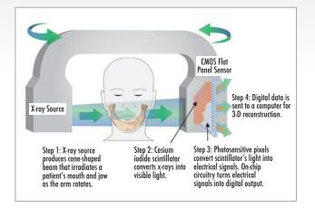
Figure 3: Conversion of in-coming X-ray photons to an electrical signal by the image detector.
