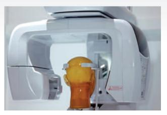
Figure 1: Basic elements of CBCT imaging hardware – X-ray source on the left, Image detector or sensor on the right, and the gantry or rotating platform that connects the x-ray source and the detector.
