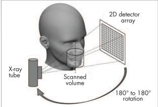
Figure 4: The x-ray source and reciprocating image detector synchronously moves 180° to 360° around the patients head.
