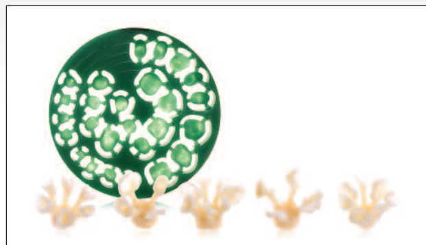
Figure 11: The individual restorations were machined in wax, pressed with lithium disilicate glass-ceramic and subsequently finished.
