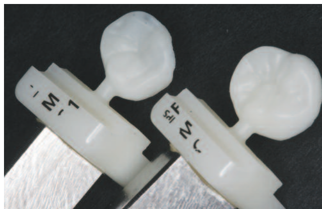
Figure 8. Milled restorations with sprue
