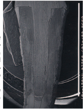
Figure 11: Half a root with a post luted inside after being directly exposed to water for 6 months. Direct exposition of the bonding interface to water determined degradation of the hybrid layer.
