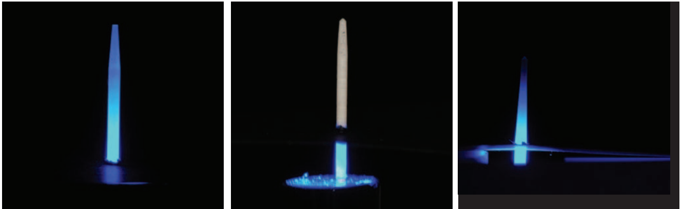
Figures 19a, 19b and 19c : Three types of posts show different penetration of light through them.
