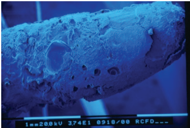
Figure 9: A post luted with all-in-one adhesive system in combination with a dual-cure resin cement: the material combination cannot cure.
