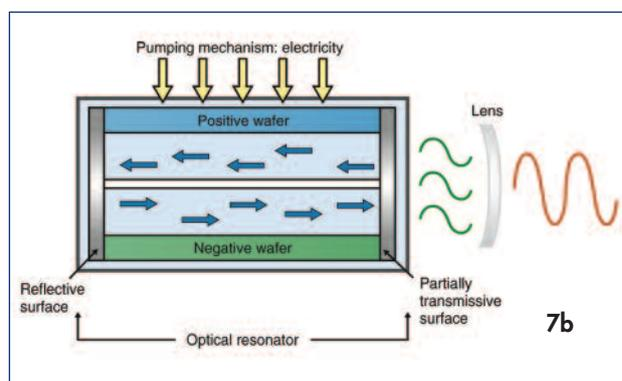
Figure 7: (a) Components of a gas or solid active-medium laser, eg. CO<sub>2</sub> or Nd:YAG laser, and (b) a diode laser. Adapted from *Principles and Practice of Laser Dentistry 2nd ed* (p. 14), by Convissar RA, 2015, St. Louis: Mosby Elsevier
