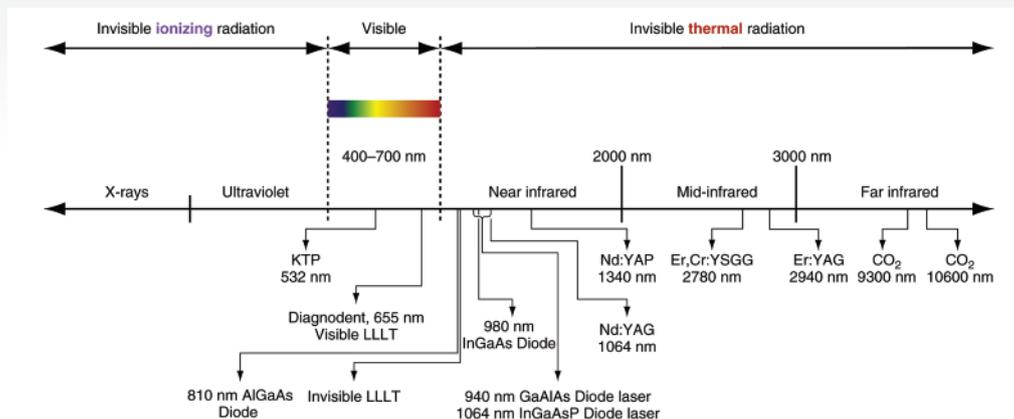
Figure 8: Wavelengths of the various laser lights and their position within the EM spectrum. Adapted from *Principles and Practice of Laser Dentistry 2nd ed (p. 14)*, by Convissar RA, 2015, St. Louis: Mosby Elsevier
