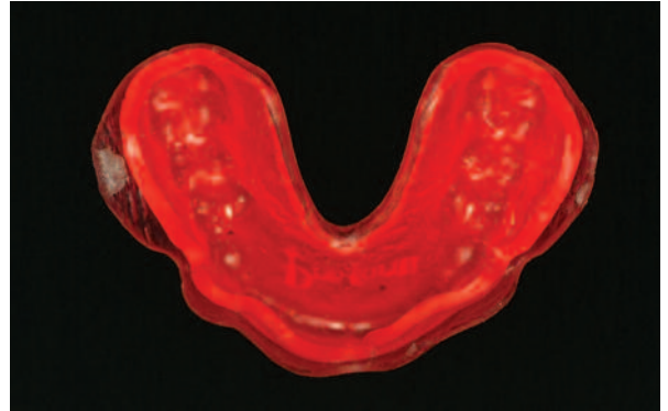
Figure 5: Vacuum forming is incapable of bonding layers of EVA together and mouthguards thus formed will often delaminate.
