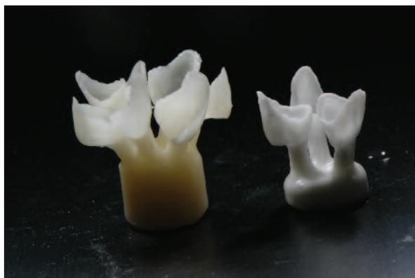
Figure 6: Translucent and opaque frameworks after pressing.
