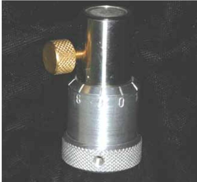
**Figure 1: Custom made cylindrical device employed for cement disks fabrication.**
