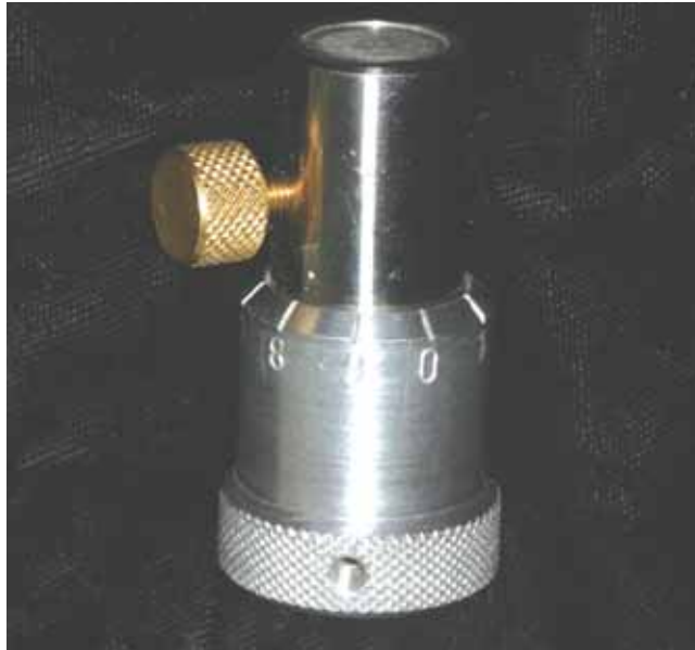
Figure 1: Custom made cylindrical device employed for cement disks fabrication.
