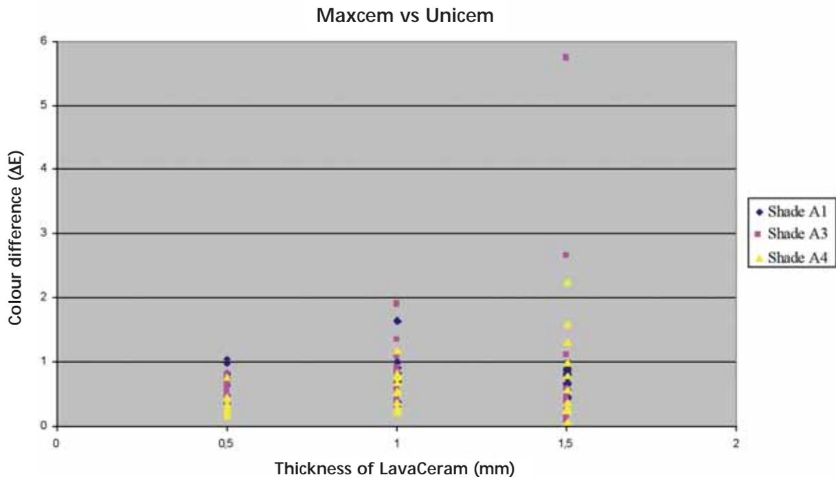
Figure 4: Colour differences ( $\Delta E$ ) between Maxcem and Unicem for samples of LavaCerem of different thickness (0,3-0,7) in shades A1, A3 and A4 on Lava cores of different thickness (0,3-0,7) and stain.
