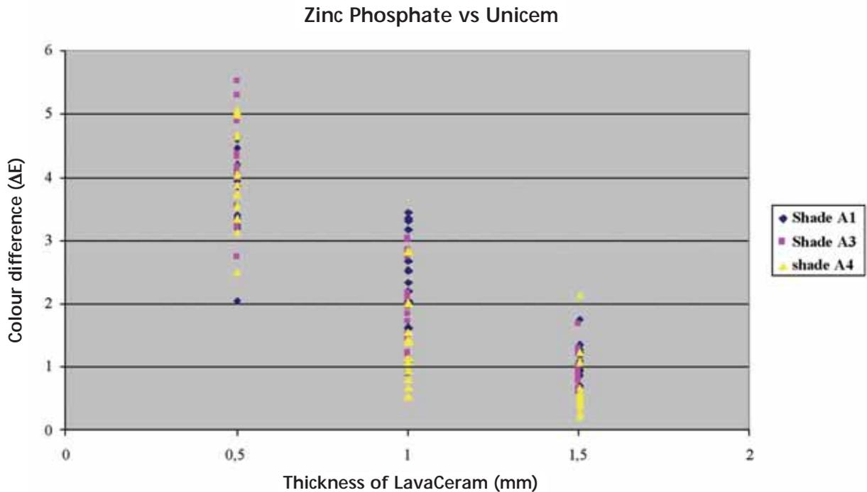
Figure 2: Colour differences ( $\Delta E$ ) between Zinc-Phosphate cement and RelyX™ Unicem for samples of LavaCeram of different thickness (0,3-0,7mm) in shades A1, A3 and A4 on Lava cores of different thickness (0,3-0,7mm) and core modifiers. Clinically significant colour variations( $\Delta E$ ) are observed when 0,5mm porcelain is used.
