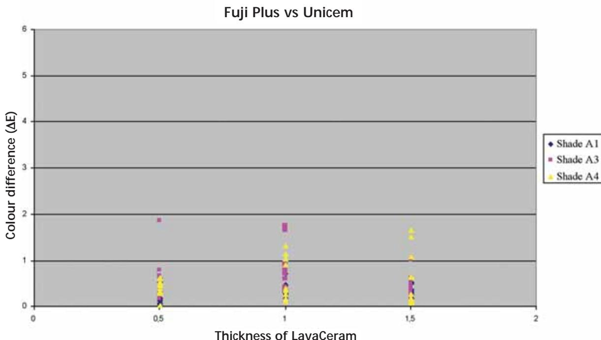
**Figure 5: Colour differences ( $\Delta E$ ) between Fuji plus and Unicem for samples of LavaCeram of different thickness (0,3-0,7) in shades A1, A3 and A4 on Lava cores of different thickness (0,3-0,7) and stain. All the colour differences ( $\Delta E$ ) observed are below the value 2.**
