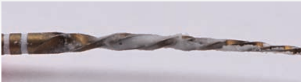
Figure 14: WaveOne® Gold Primary after the first cutting cycle. Note the flutes are filled with cutting debris.
