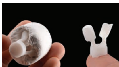
Figure 7: The pressing gives a homogeneous result, and barely any reaction layer is formed.
